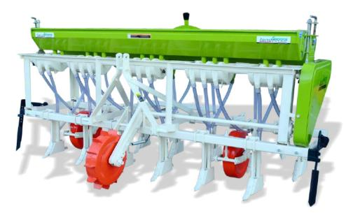
Landforce seed cum fertilizer drill is used for simultaneous activities of Seeding and Fertilization process in a single operation. It can be retrofitted to a tractor of 35 HP and above. It drill seeds and fertilizer together but delivers them separately in a single drive. Seed and Fertilizer are drilled at different depths thus improves germination. there are separate containers for seed and fertilizer.
