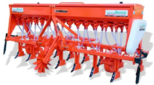
Landforce seed cum fertilizer drill is used for simultaneous activities of Seeding and Fertilization process in a single operation. It can be retrofitted to a tractor of 35 HP and above. It drill seeds and fertilizer together but delivers them separately in a single drive. Seed and Fertilizer are drilled at different depths thus improves germination. there are separate containers for seed and fertilizer.
