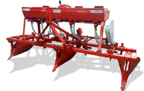
Multi Crop Raised Bed Planter is used for sowing bold grains like maize, groundnut, peas, cotton, sunflower etc. On the raised bed formed by ridgers. The planting discs for different crops can be changed without dismantling the seed hoppers main shaft. Missing of grains and grains damage is negligible. Fertilizer can be used simultaneously according to requirement. Roller is provided for shaping the raised bed properly and covering the seeds.
