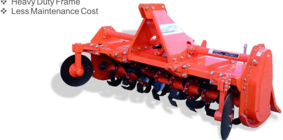
A Robust design and ultimate tillage technology suitable for hard, black cotton and rocky soil. Heavy duty gear box and frame makes it strong for rough and tough conditions. The working depth can be adjusted by the height of the skids, which is easily done with the adjustment bracket on the Rotary Tillers.
